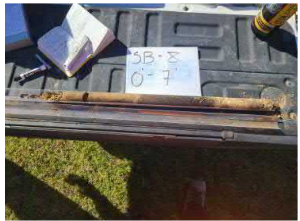
Photo 2: Additional representative view of a soil boring core
