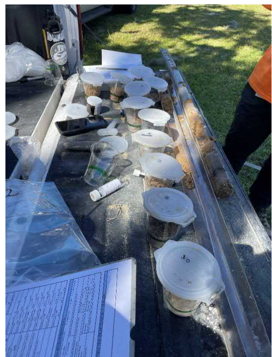
Photo 4: Representative view of soil screening procedure
